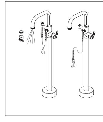
After Installationis complete remove the aerator with the provided aerator key and flush the water lines. Turn on the hot and cold supply lines and allow water to flow for approximately 1 minute. After flushing re-insert the aerator.
