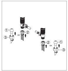
Connect the hoses (2) to the bottom of the hot and cold end valves (1 & 3), as shown. Carefully bend the hoses (2) to fit in the available space, and carefully thread the hose (2) couplings onto the sides of the connector (4) of the spout assembly. Tighten all connections with a wrench.
