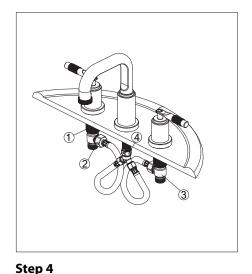
Connect the hoses (2) to the bottom of the hot and cold end valves (1 & 3), as shown. Carefully bend the hoses (2) to fit in the available space, and carefully thread the hose (2) couplings onto the sides of the connector (4) of the spout assembly. Tighten all connections with a wrench.
