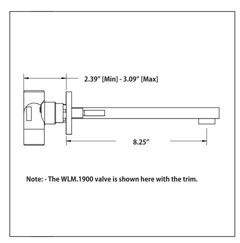
Install a crossbeam at the location where the valve will be installed. The distance between back of the valve to the finished tile surface should be between 2.39" and 3.09".
